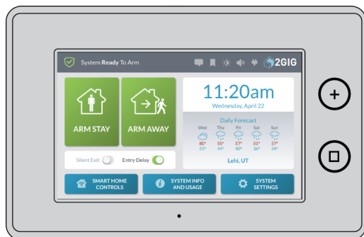
Figure 1 GC3 Control Panel—Front View
